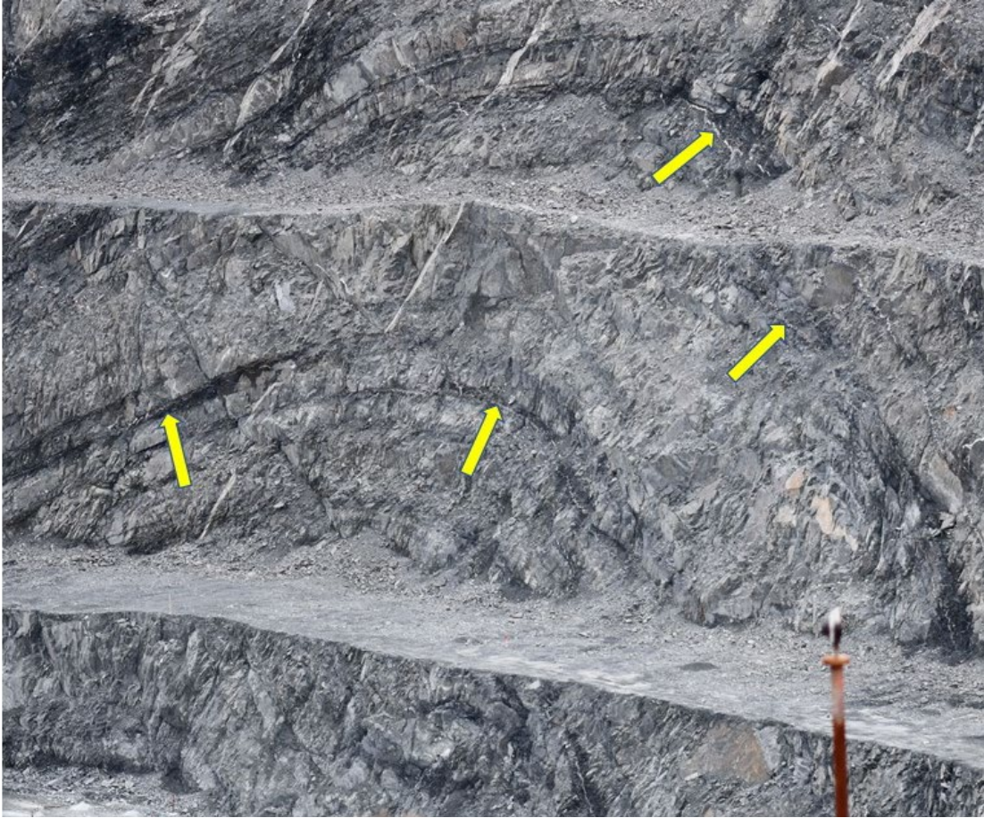
Figure MR4: Close-up photograph of the anticline hinge in the Touquoy deposit showing several strongly buckled bedding-concordant veins (yellow arrows).
