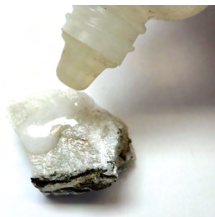
Weak hydrochloric acid reacting with calcite.
