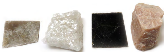
Typical colours of common minerals: From left to right, grey-white muscovite mica, milky quartz, black biotite mica, and pale-orange orthoclase feldspar.
