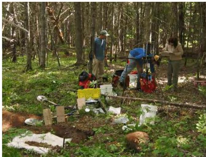
*Field sampling for the NASGLP project in northern New Brunswick. In the foreground is a soil pit and sampling gear with buckets and an auger. A soil permeability meter and radon measurement kit is in the background. Photograph: Mike Parkhill.*
