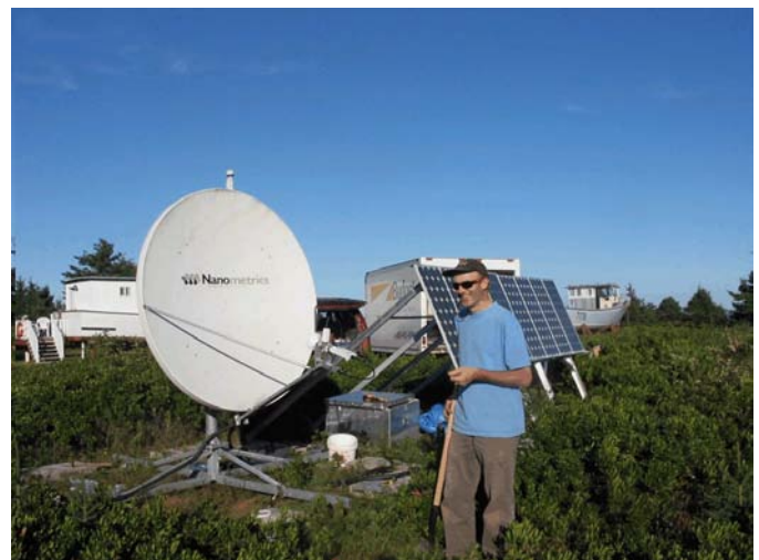
Patrick Potter enjoys a sunny day last Fall during set-up of ARTE seismometer network. The solar panels on the right power the seismometer and satellite dish for real-time transmission of the ground-motion data (photo: Sonya Dehler).
